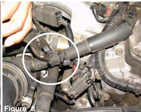
Figure 8 Using a set of pliers, depress the tension clamp on the hose and pull the clamp away from the air intake port.
