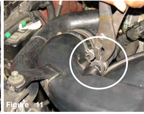
Figure 12 The air bypass line is disconnected from the air intake port.
