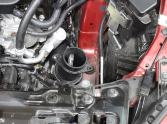
27. Place the left side (Driver) bracket into the rubber grommet on the frame rail. The top of the support bracket will sit just under the MAF housing mounting ear. Clock the silicone coupler and MAF housing so that the bracket perfectly aligns with the mounting ear. At this point, tighten the #32 hose clamp on the turbo inlet locking the coupler in place.
