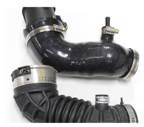
**15.** Install the silicone coupler in the car. First attach the PCV vent hose using the smaller OEM clamp. Then fully install the coupler onto the turbo inlet. Do not tighten the hose clamp yet.
