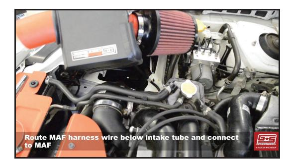
18. Get the heat shield assembly into position and then push the intake tube down towards the fender to ensure that you have plenty of slack in the MAF harness wire. At this point, go ahead and use the rubber grommet and heat shield slot from earlier to safely secure the MAF wire.
