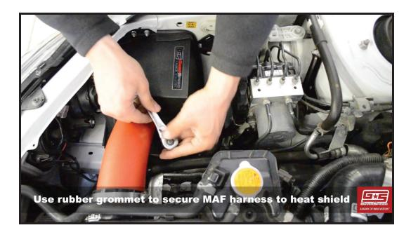
20. Reinstall the two 10mm nuts to secure the heat shield to the vehicle using a 10mm socket.
