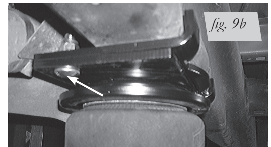
Right hand assembly (passenger side) attached with carriage bolts (R), flat washers (M) and nylon lock nuts (U). Torque to 31 lb.-ft.
