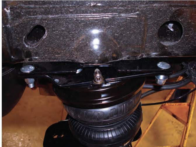
Driver-side (left) assembly shown. NOTE: Fitting goes on the outside of the frame.
