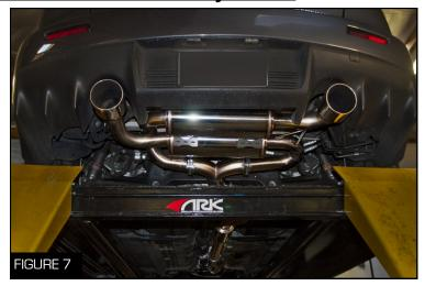
10. While one person properly aligns the tips, the other person should bolt down each nut and bolt to the proper torque specs (Figure 7)
