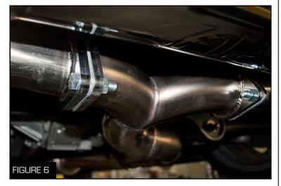
9. Bolt the muffler and Y-pipe together with the supplied gaskets and hardware using both 14 and 17 mm socket wrenches (Figure 6)
