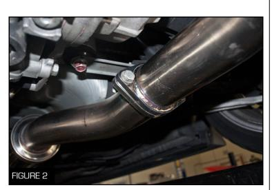
supplied gasket and hardware using both 14 mm and 17 mm socket wrenches (Figure 2)
