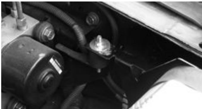
Align the Power box bracket to the vibra-mount stud and use the m6 nut and fender washer to secure the box in place.
