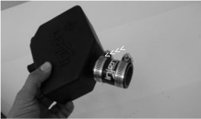
Take the CCV connecting hose and press it over the CCV box port. Use the two small clamps to hold the hose in place and tighten the clamp on the port side.
