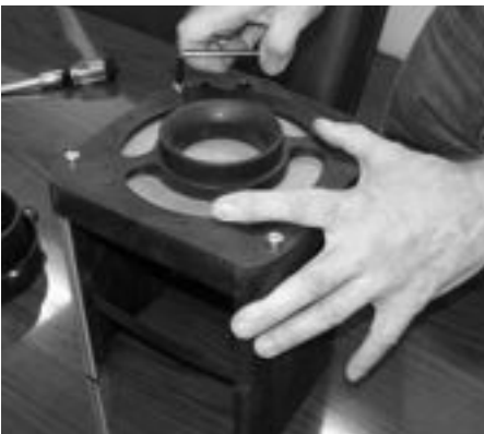
Unbolt the four-45mm screws from the Power-box top. The screws are located towards the corners of the top.
