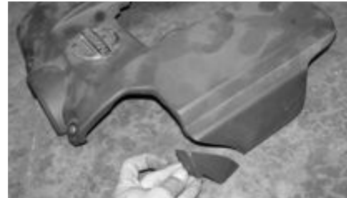
Use a utility knife to cut a small corner section as shown in this picture. Cut small sections at a time until a perfect fit is achieved,
