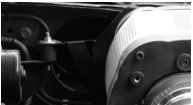
Here is a side view of the Power box bracket connected to the vibra-mount stud.
