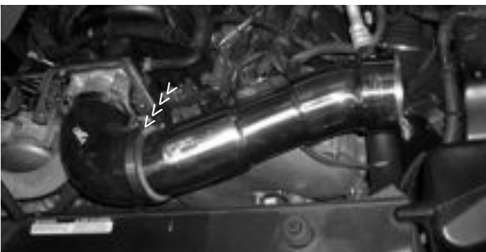
Take the assembled intake and press the 3 1/2" end into the silicone elbow. Do not tighten clamp located on the silicone elbow.
