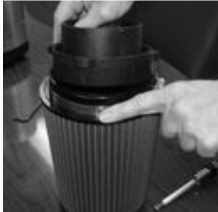
Once the clamp has been loosened, gently separate the velocity stack from the filter neck.
