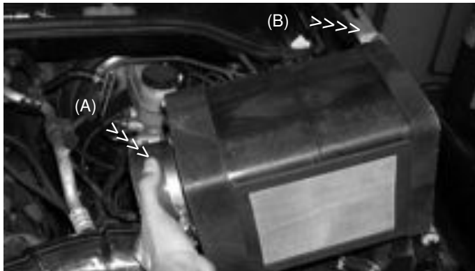
The assembled Power box is lowered into the engine compartment. The 4 inch hose is pressed over the end of the intake (A) and the Power box bracket is lined up to the vibra-mount stud (B).
