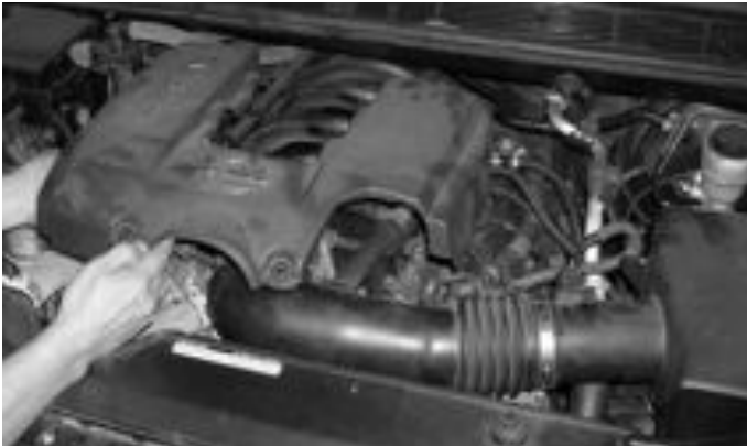
Unbolt the two front screws and remove the plastic cover located over the intake manifold.
