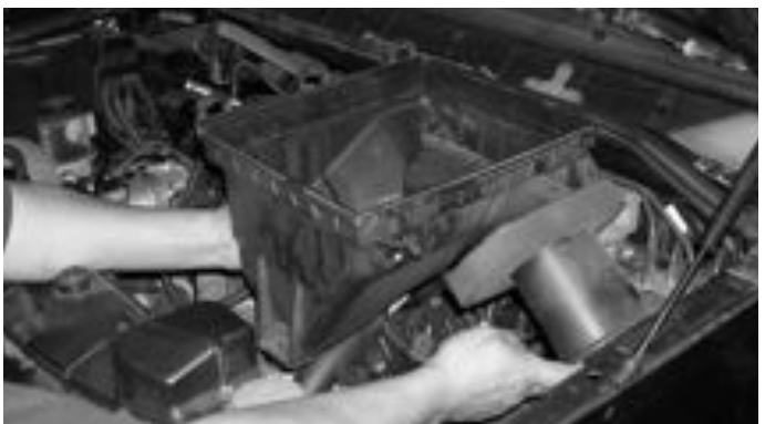
Remove flat filter panel from the filter box. Once filter has been removed, gently pull lower box out of the stock location.
