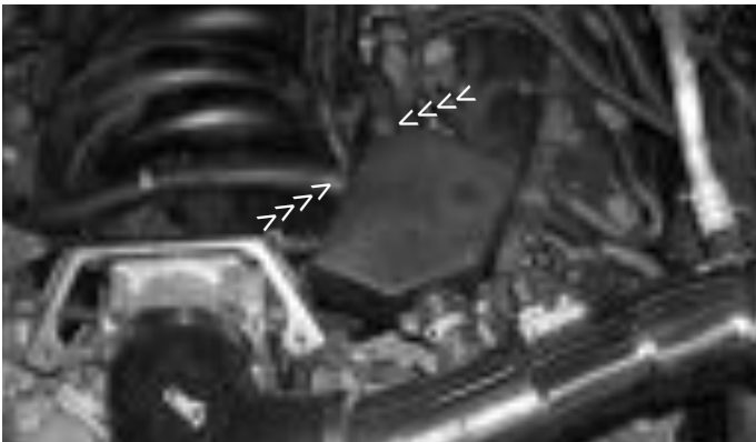
The driver and passenger side crank case breather lines are now connected to the CCV box.
