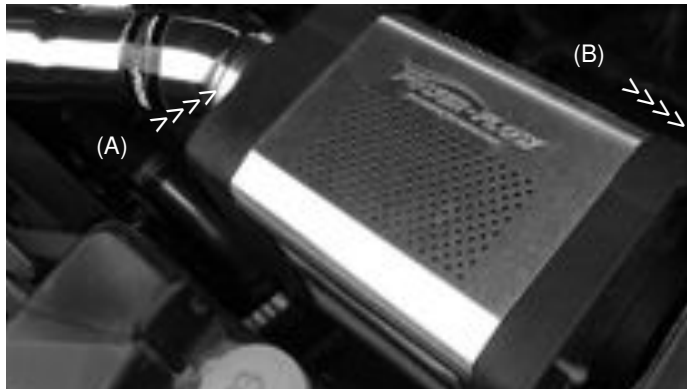
The Power box velocity stack base is connected to the intake (A) and the Power box bracket is lined up to the vibra-mount stud (B).
