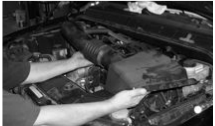
Remove screws, loosen clamps and remove upper air intake box and air intake duct connected to the throttle body.
