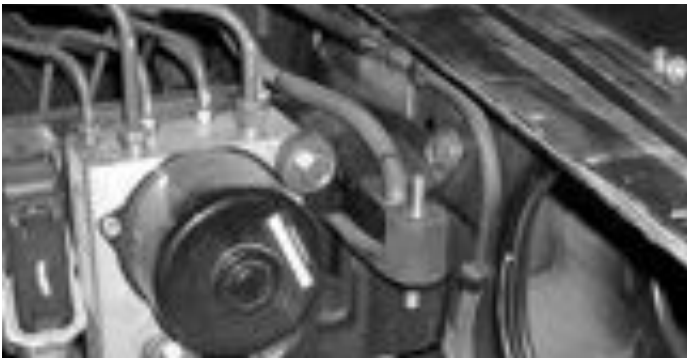
Find brace located in front of the ABS solenoid and screw vibra-mount into the brace until it bottoms out.
