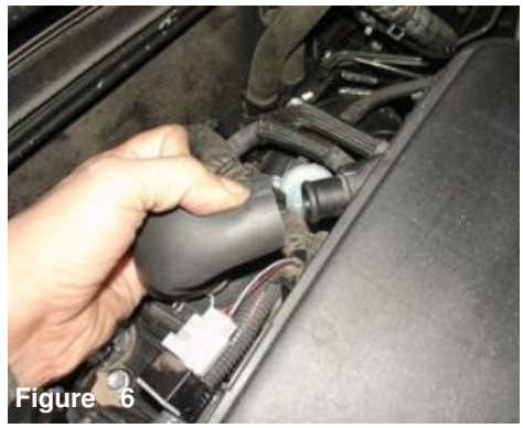
Figure 3 Disconnect the MAF sensor harness. Pull all lines away from the stock air box system.
