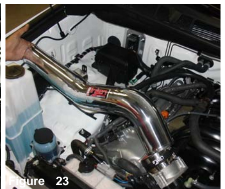
Figure 23 Install intake into vehicle and position.
