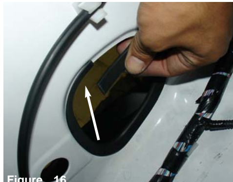
Figure 16 Attach the vinyl trim to hole cut out on fender well.
