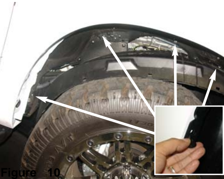
Figure 10 Remove all the plastic clips holding in splash guard under passenger side fender well. Pull down splash guard.
