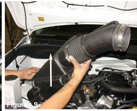
Figure 9 Lift up and pull out complete stock intake system out of vehicle.
