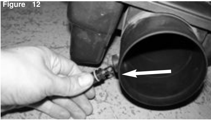
Carefully turn then pull out the temperature sensor out of resonator box.
