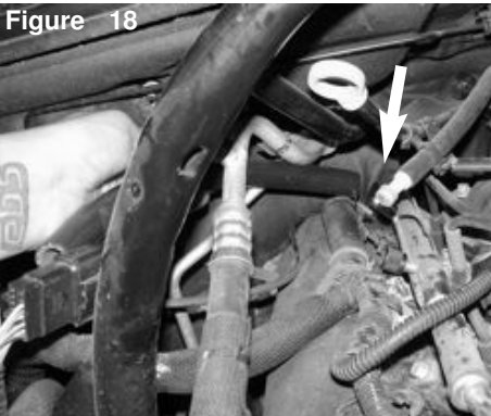
Install the new provided 15mm hose to the fitting on engine side.
