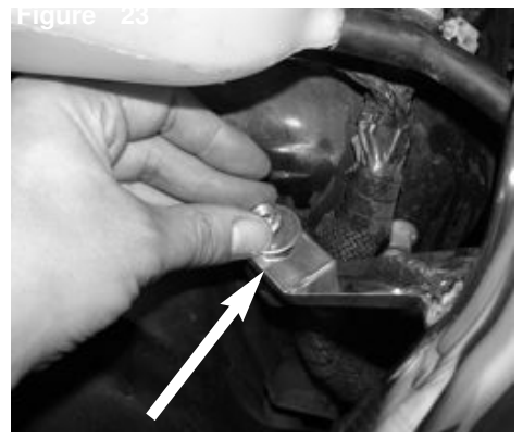
Figure 23 Secure the bracket using M6 nut and washer.
