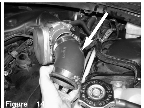
Figure 10 Install the longer side of the vibra mount to the engine valve cover.
