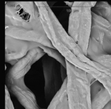
Existing media without Injen SuperNano-Web Technology
