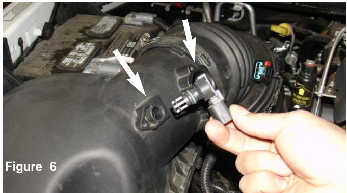
Figure 4 Depress the tab on the electrical harness clip and disengage it from the MAF sensor and temperature sensor.
