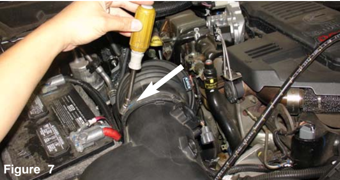
Figure 5 Use a 8mm nut driver to loosen the 3 screws holding in MAF sensor and temperature sensor.
