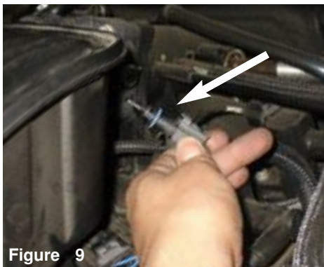
Figure 6 Pull back the crank case line from the air box.
