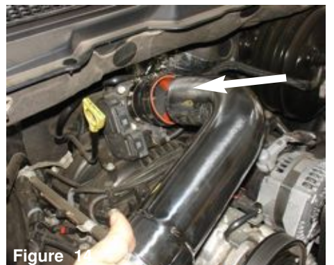
Figure 11 With provided M8 vibra mount install to the threaded fitting located on the fender frame next to air box bracket.
