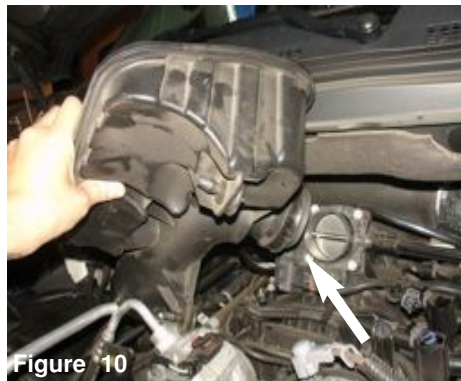
Figure 7 Now carefully lift up the air box assembly and remove from the engine compartment.
