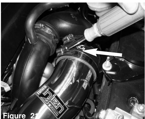
Figure 22 Reconnect the temp sensor harness.
