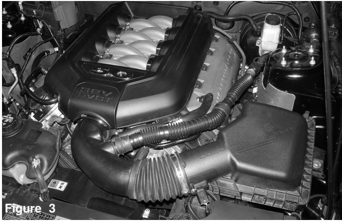
Figure 3 Complete stock intake shown. Disconnect battery before install.
