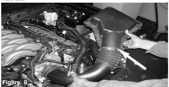
Figure 8 Carefully lift up and pull out the stock upper half of air box from vehicle.
