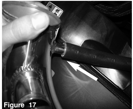
Figure 14 With clamps provided, install the 3-1/2" straight hose to the throttle body.
