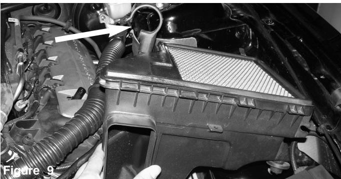
Figure 9 Carefully lift up and pull out the bottom air box from vehicle. Make sure that the sound tube rubber isolator is disconnected.
