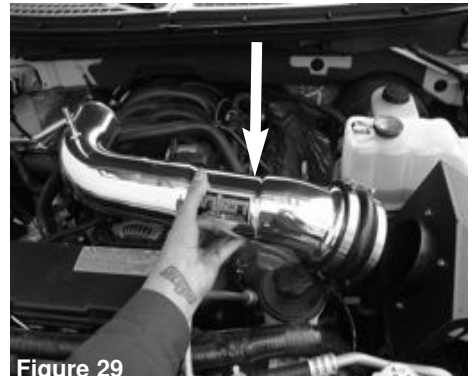
Figure 29 Install the intake tube into the vehicle and position to the throttle body and adaptor.
