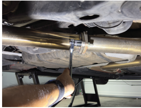
2. Remove the two nuts securing the mid pipe to the OEM muffler section.
