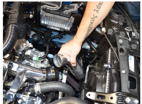
33. Install the secondary cold side intercooler pipe. Insert the pipe into the bottom hose then into the top hose.
