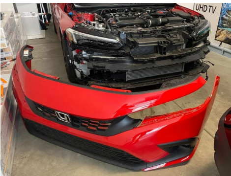
7. Remove the front bumper. Refer to the honda service manual for instructions.
