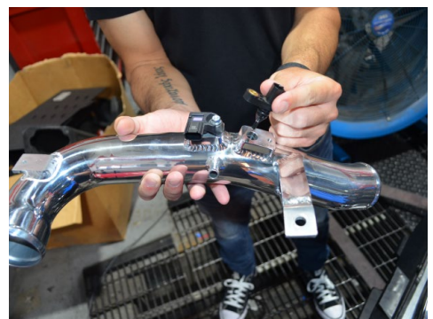
24. Install the pressure and temp sensor onto the injen cold side primary intercooler pipe. Secure both with the OEM bolts.
