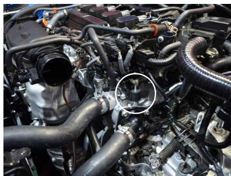
23. Install the provided M6 Vibra mount onto the threaded hole on the thermostat housing.
