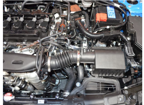
42. Ensure all nuts, bolts and clamps are properly secured, then ensure all harnesses and vacuum lines are connected.
