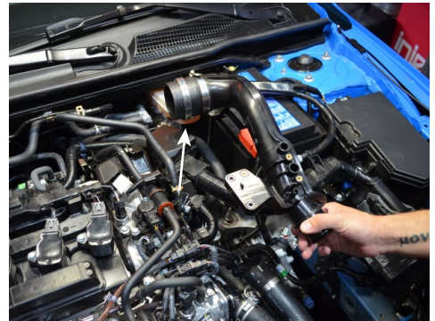
18. Loosen the clamp securing the intercooler pipe to the throttle body, then remove the intercooler pipe
