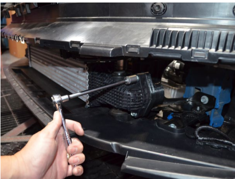
31. Secure the intercooler adapter to the outlet on the intercooler using the OEM bolts
