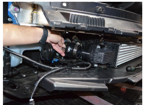
36. Install the 2.25" hump hose onto the intercooler adapter. Only secure the clamp on the intercooler adapter.
