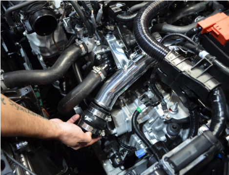
28. Install the 2.25" hump hose with clamps onto the intercooler pipe. Leave the clamps loose.
