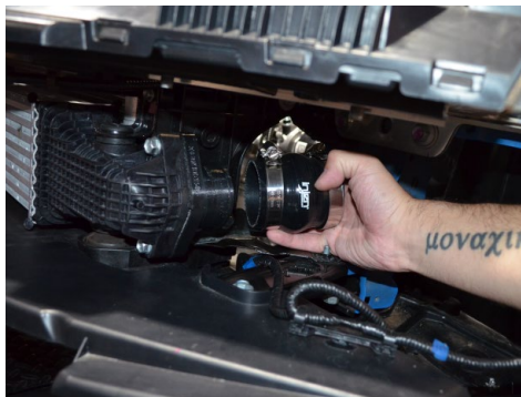
32. Install the 2.25" hump hose onto the intercooler adapter. Only secure the clamp on the intercooler adapter.
