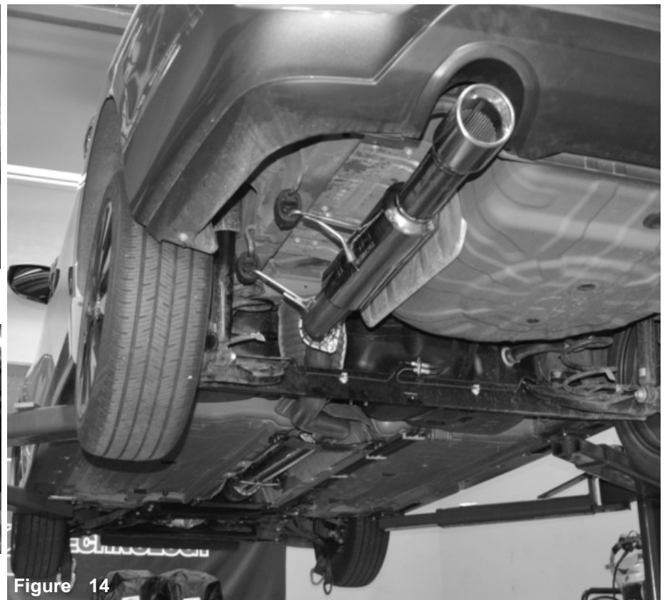
Figure 11 Install the mid section. Install the hanger to the rubber isolation mount. Connect the mid and front section using M10 bolts and nuts with gasket. Do not tighten.
