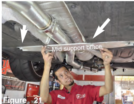
Figure 21 Re-install the mid support brace. Secure and tighten. Once completed, adjust the mid pipe to have clearance and make sure the pipe does not come into contact with the brace.
