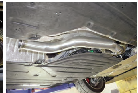
Figure 17 Adjust and set into position. Do not tighten. Note: Exhaust system has room for adjustment, re-position and tighten for best fit.
