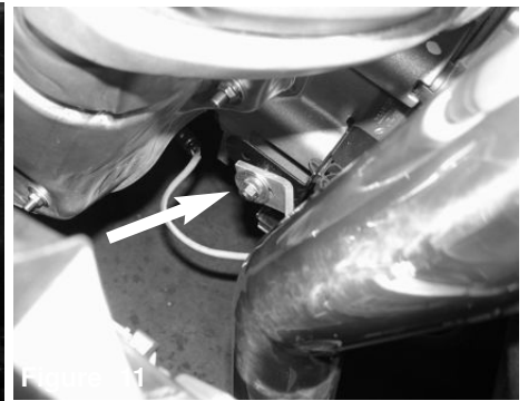
Figure 8 A) Remove the screw holding in the temp sensor using T30 torx bit B) Remove the temp sensor.
