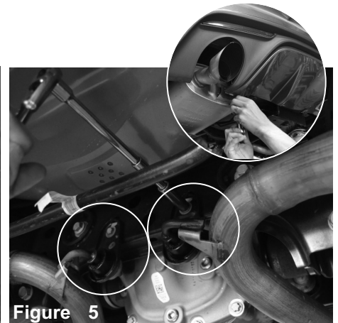
For easier removal, loosen the 13mm bolts holding in the exhaust rubber isolation mounts. Remove the rear muffler isolation mounts also using 13mm socket and ratchet.
