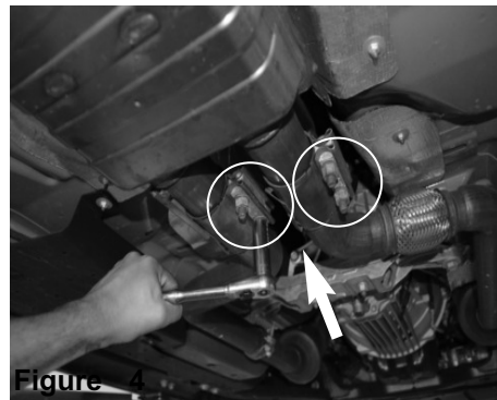
Loosen the 2 15mm nuts on both band clamps on exhaust at cat back. Loosen and pull back.
