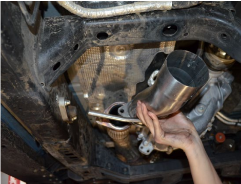
4. Connect the front pipe to the OEM flex pipe, then insert the hanger to the rubber insulator. Secure using the OEM fasteners.
