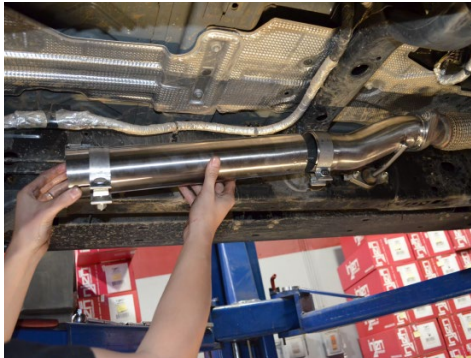
5. FOUR DOOR MODELS ONLY: Attach the mid pipe extension to the front pipe. Secure using the provided 76mm clamps.
