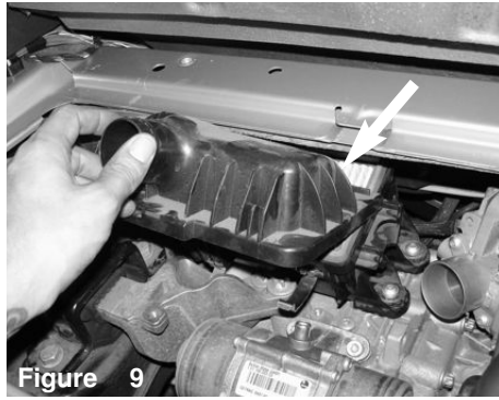
Figure 6 Using a T30 torx bit, loosen the bolt holding in the stock air box located in back of the engine close to the exhaust.
