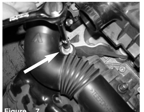
Figure 7 Loosen the remaining bolt close to the air box and remove.
