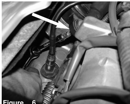
Figure 6 Using a T30 torx bit, loosen the bolt holding in the stock air box located in back of the engine close to the exhaust.
