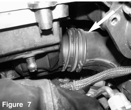
Figure 6 Pull back the MAF sensor housing from the air box.
