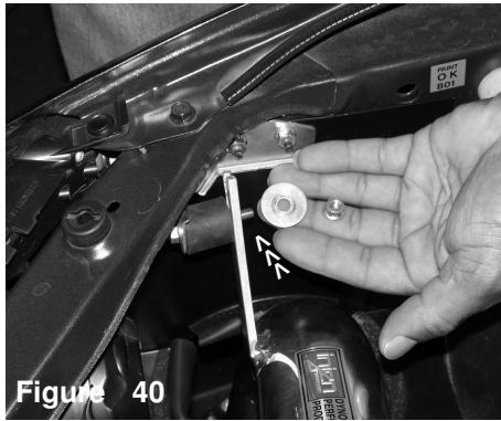
Figure 40 The m6 flange nut and fender washer is used to fasten the intake bracket to the vibra-mount stud.
