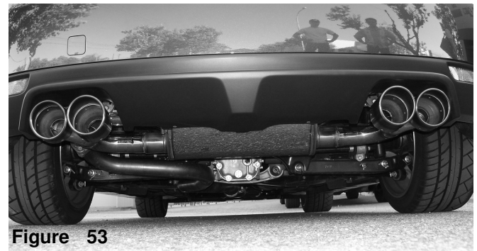
Figure 53 Injen Technology, will soon be releasing the most aggressive axle-back system on the market. While adding 16 H/P to your STi, this system features the first 4" quad titanium tips with rolled edge that adds strength. The tips come with classic burnt blue process on the end of the tips that will make you the envy of the road.
