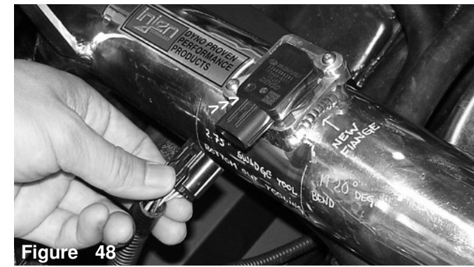
Figure 48 The electrical sensor harness is pressed over the mass air flow sensor until it snaps in place.
