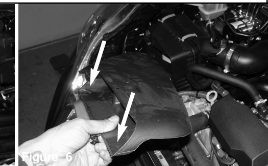
Figure 6 Remove the two plastic retaining clips indicated by the arrows and then remove the front air scoop.
