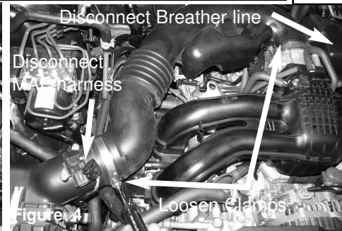
Figure 4 Disconnect the MAF sensor harness, breather line and the two clamps on the factory intake air duct.
