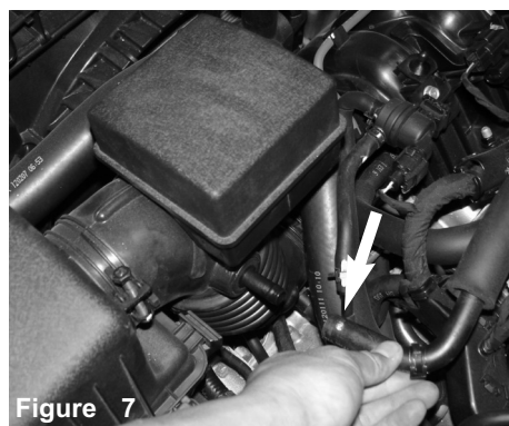
Figure 7 Disconnect the crank case vent tube from the air box duct hose.
