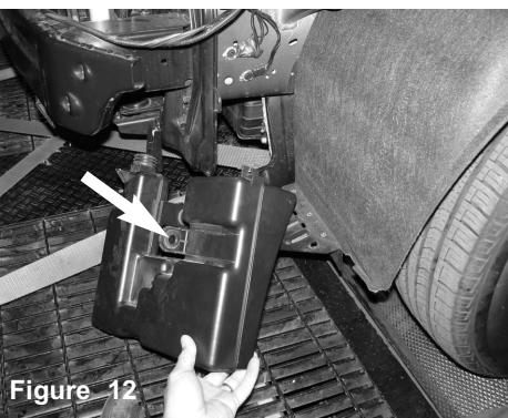
Figure 12 Locate the air box resonator in the drivers side front bumper wheel well area. Remove the 10mm bolt attaching the resonator to the chassis and then pull the entire air box resonator out.
