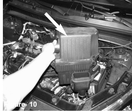
Figure 10 Lift up on the air box assembly and remove the entire air box assembly from the engine bay.
