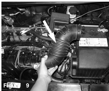
Figure 9 disconnect the air duct from the throttle body and air box and remove the air duct hose
