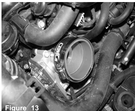
Figure 13 Place the 2.75" straight hose and two #40 clamps onto the throttle body and only secure the clamp on the throttle body side only for now.
