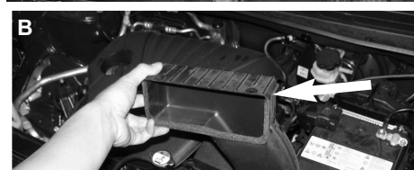
Figure A: Use a phillips screw driver and remove the two plastic retaining screws on the front vent duct. Figure B: This air duct will be removed.
