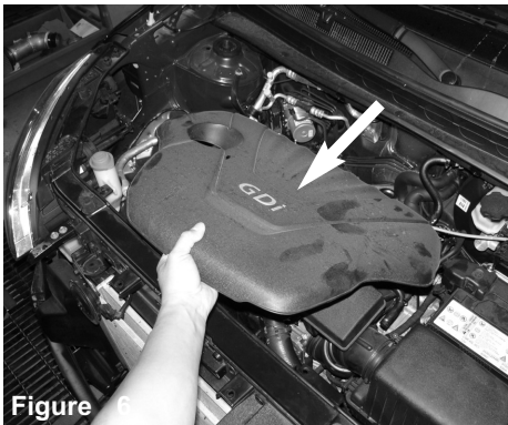
Figure 6 Firmly lift up on the engine cover and remove the engine cover from the engine bay for now. This cover will be re-installed later
