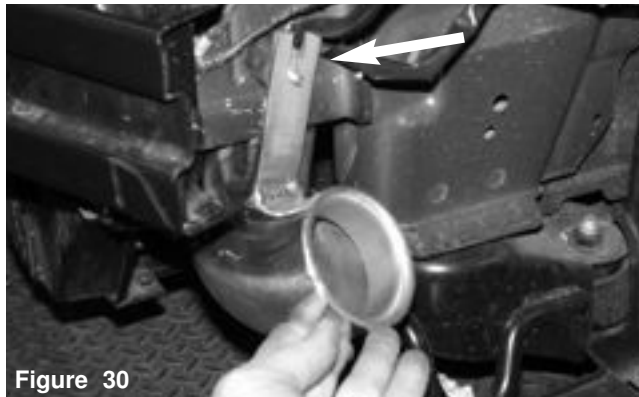
Figure 28 Slide the intake pipe from the bottom and work the pipe into the 90 deg. hose already located on the throttlebody.
