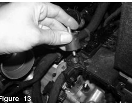
Figure 13 Install the vibra mount to the factory threaded fitting where the air box mounted to. Secure and tighten.
