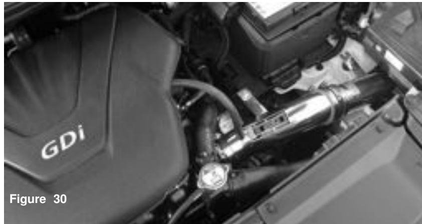
Figure 28 Attach the crank case hose to the fitting on the intake tube and secure. Re-install the front bumper cover and re-connect the battery.
