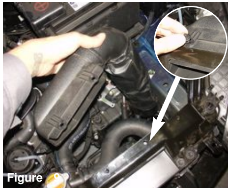
Figure 6 With 10mm socket and ratchet loosen the 3 screws holding in the air box assembly.
