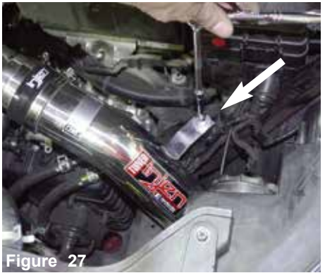
Figure 27 Now tighten the nut using 10mm socket and extension.
