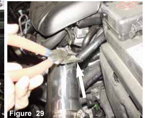
Figure 29 Secure using the factory clamp. Re-install bumper cover and connect battery terminals.
