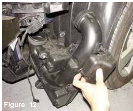
Figure 12 Pull any lines that are attached on or the resonator and remove from the vehicle.
