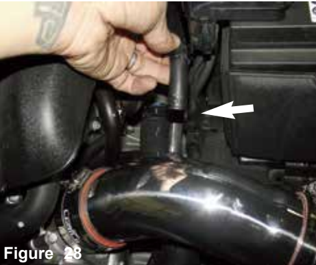
Figure 28 Now secure the crank case line to the fitting on the intake tube.
