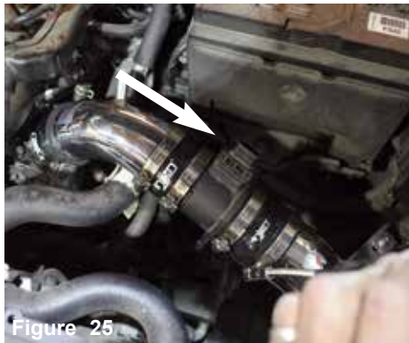
Figure 25 Position for best fit and tighten the remaining clamp using 8mm nut driver.
