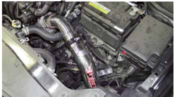
Figure 29 Secure using the factory clamp. Re-install bumper cover and connect battery terminals.
