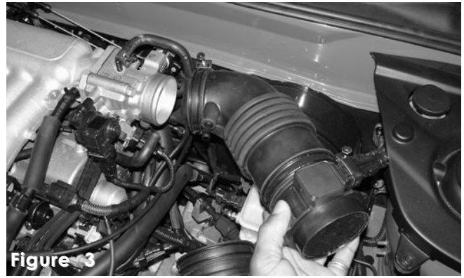
Once the clamp has been loosened from the throttle body and the air box cleaner, continue to remove the mass air flow sensor and air intake duct from the throttle body.
