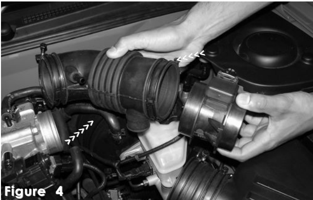
Once you have removed the entire air intake duct, continue to loosen clamp on the plastic air duct from the inlet side. Continue to pull the mass air flow sensor from the air intake duct.
