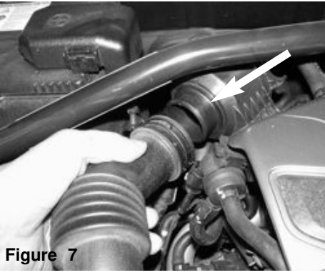
Figure 7 Pull back the sound tube from the resonator. Disconnect the brake booster line if equipped.
