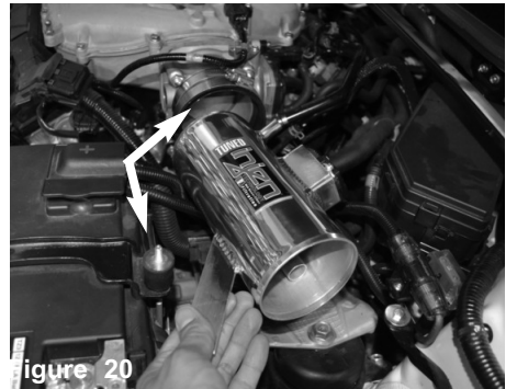
Figure 17 For cold air application install the m6 vibramount to the OEM air box mounting insert.
