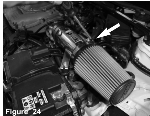
Figure 21 Secure and tighten the clamps. Tighten the bracket on the vibramount.
