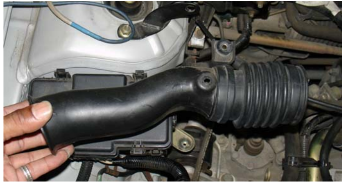
Remove the stock air intake duct connected from the box to the throttle body.
