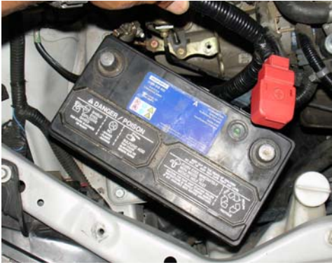
For this installation remove the negative and positive battery terminals, then proceed to remove the battery. Always place the battery on a table or cardboard paper in order to prevent grounding of the battery.
