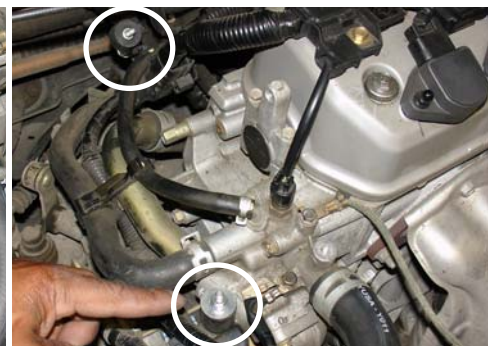
Both vibra-mounts are now installed and ready for the next step.
