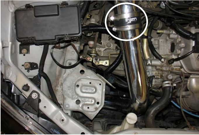
Once the bracket has been aligned to the vibra-mount stud press the upper end of the intake into the 3" hose on the primary intake.
