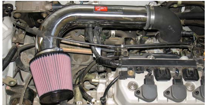
The filter is pressed over the end of the primary intake and used as a short ram. Injen recommends using the short ram in rainy days in order to avoid hydrolocking.
