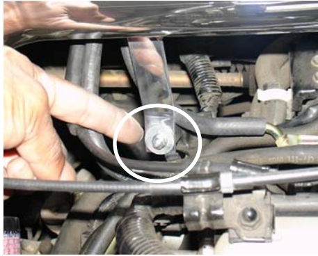
While the intake is pressed into the silicone elbow the bracket is lined up the the first vibra-mount stud, as shown above. Use the m6 flange nut and fender washer to hold the intake in place.
