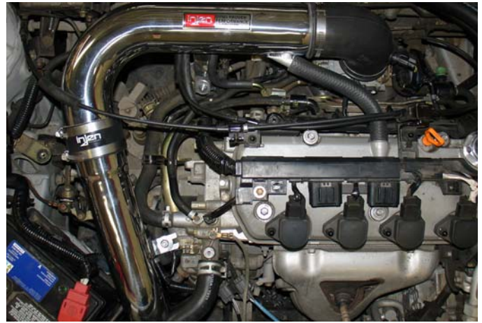
Once the entire intake has been installed continue to align the intake for best possible fit. After proper clearance has been made through out the length of the intake continue to tighten all nuts, bolts and clamps. Periodically check the alignment of the intake tract in order to avoid damage to the intake system.
