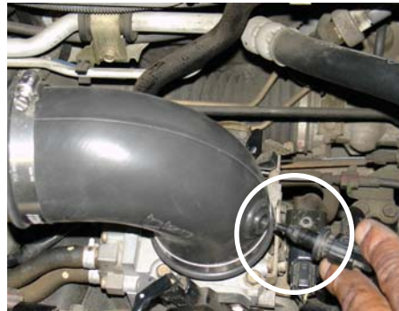
Take the air temperature sensor and press it into the grommet placed in the 90 degree elbow.
