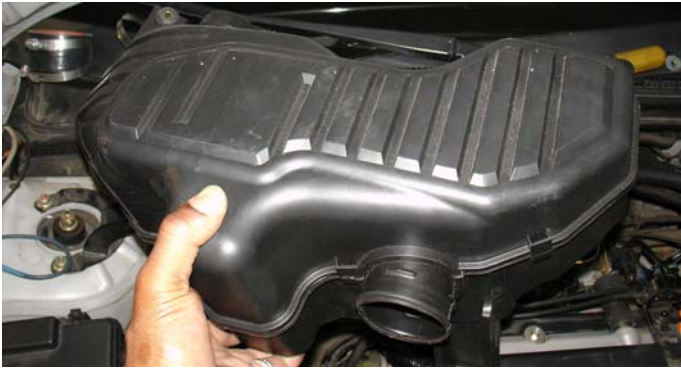
Disconnect any vacuum lines connected to the stock air box and remove the stock air intake box from its stock location
