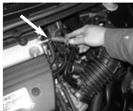
Figure 7 Now remove the rubber line connected to the CCV port on the valve cover.
