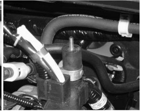
Screw the vibra-mount into the air box stud until it bottoms out.
