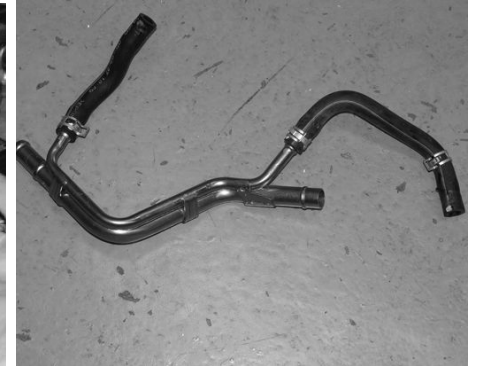
The PCV hard pipe is now removed from the engine compartment intact.
