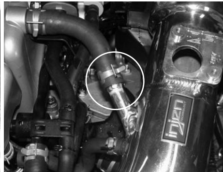
The crank case breather hose is shown connected over the 1/2" intake port. The stock clamp is used to hold the stock hose over the intake port.
