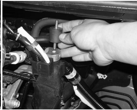
Align the vibra-mount over the air box stud as shown above.
