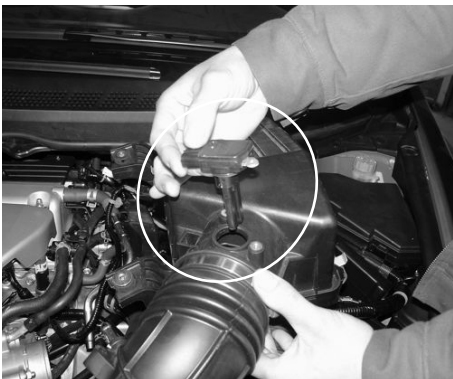
Remove the two screws holding the mass air flow sensor to the air intake duct. Gently pull the mass air flow sensor from the air intake box as shown above.
