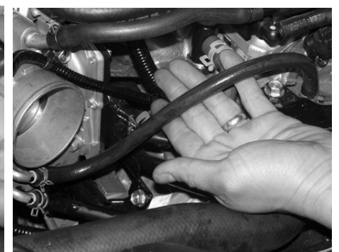
The 12"- 6mm vacuum hose is connected to the upper coolant out port and the throttle body coolant port.
