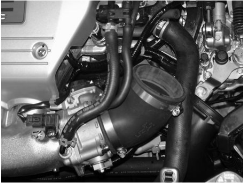
Press the 2 3/4" end on the 45 degree elbow over the throttle body. Use two power-bands and semi-tighten the elbow over the throttle body.
