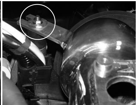
Align the intake bracket to the vibra-mount stud. Use the fender washer and m6 flange nut to secure the intake to the vibra-mount.
