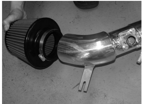
Carefully, insert the 3 1/2" filter neck over the end of the intake.
