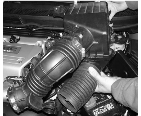
Loosen the clamp on the throttle body and gently pull the air intake box, and both air intake ducts out as shown above.
