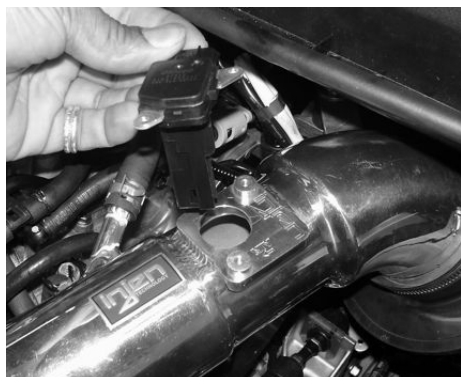
Gently, press the mass air flow sensor into the machined adapter as shown above. Place a dab of light oil around the sensor O-ring. This will allow an easy and good seal between the adapter and O-ring.
