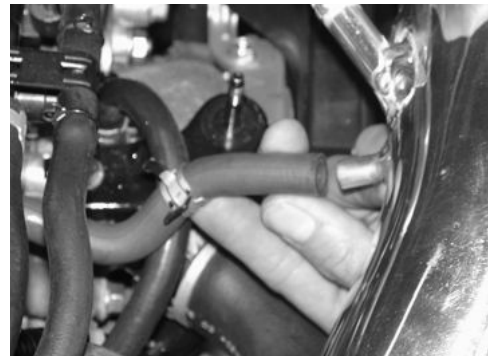
Press the air control thermal hose over the 3/8" intake vacuum port as shown above. Use the stock clamp to secure the hose in place.
