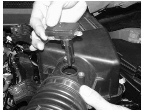
Remove the two screws from the mass air flow sensor top.
