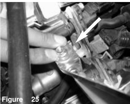
Figure 22 Using the factory screws, secure the MAF sensor.
