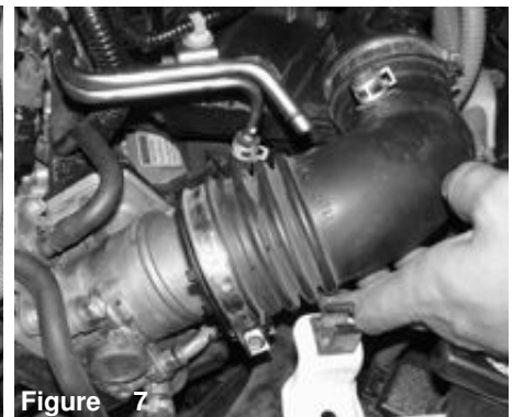
Figure 4 With pliers, loosen the mini clamp holding in the crank case line.
