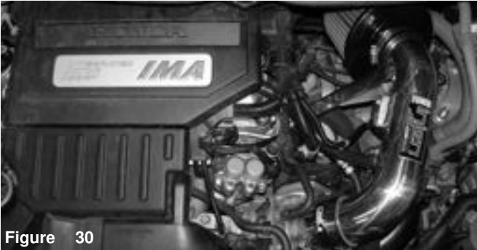
Align the entire intake for the best possible fit. Once you have rechecked and cleared the intake from all moving parts, continue to tighten all nuts, bolts and clamps.
