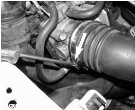
Figure 5 Loosen the clamp on the throttle body using phillips screwdriver.
