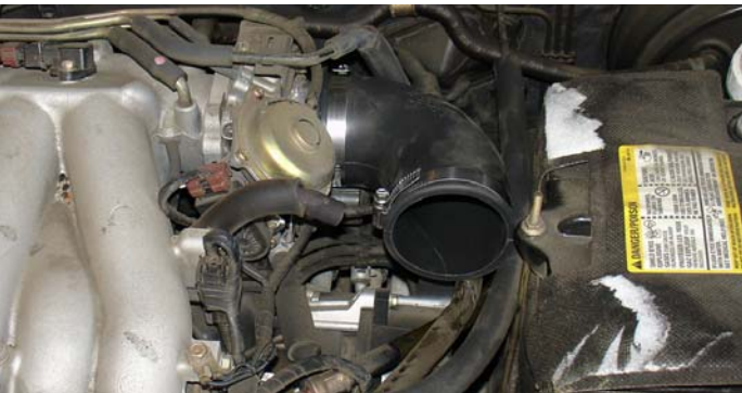
Take the 90 degree elbow and press the end with the velocity stack over the throttle body. Place a medium clamp (.048) on each side of the elbow and semi-tighten the clamp on the throttle body side.
