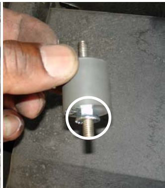
Take one of the 6mm flange nuts and place it on one end of the vibra-mount until it bottoms out.
