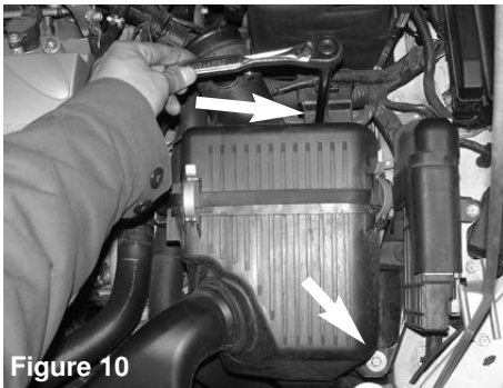
Figure 7 Detach the air duct from the air box assembly
