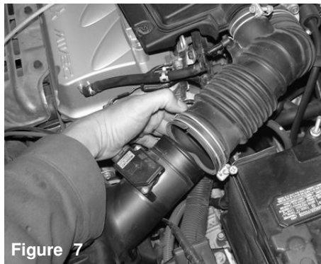
Figure 4 Loosen the clamp on the intake air duct attached to the throttle body
