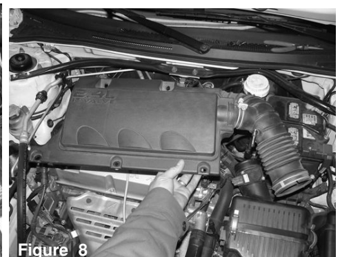
Figure 7 Detach the air duct from the air box assembly
