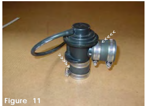
Figure 11 Press the new reinforced short hose over each port on the blow-off valve. Use the .020 mini clamps provided in this kit to secure the hose in place.
