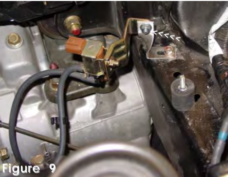
Figure 9 Mount the boost control solenoid bracket to the 1450T bracket. Use an m6 x m16 hex bolt and flange nut.
