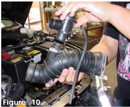
Figure 10 Remove the blow-off valve from the stock intake duct.
