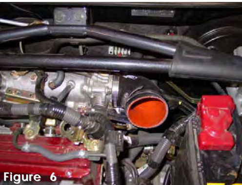
Figure 6 Press the 90 degree elbow on the throttle body and use two .312 power-bands on the elbow. Semi-tighten the clamp on the throttle body at this time.
