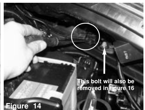
Figure 14 Remove the plastic clip underneath the drivers side headlight that is attached to the resonator tube. This bolt will also be removed in figure 16
