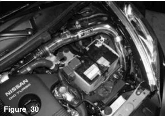
Figure 30 Congratulations! You have just completed the installation of this intake system. Periodically, check the alignment of the intake, normal wear and tear can cause nuts and bolts to come loose. Failure to check the alignment and adjust the intake can cause damage that will void the warranty.
