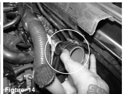
Figure 14 Install the 2" straight hose to the turbo using clamps provided. Tighten the clamp on the turbo only using 8mm nut driver.
