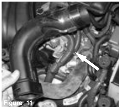
Figure 8 The resonator tube is now detached from the CCV box.
