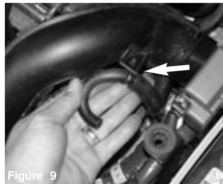
Figure 6 Pull the air resonator box from the side stand-off and remove the resonator box.
