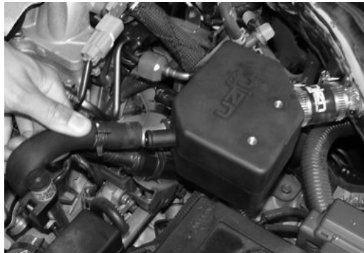
Take stock breather hose and insert it over the open CCV box port as shown above.
