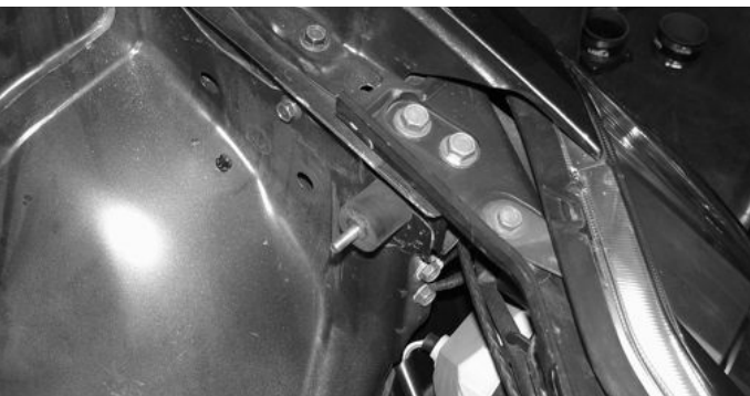
Take the vibra-mount and screw it into fender wall. Turn the vibra-mount into the fender wall until it bottoms out.
