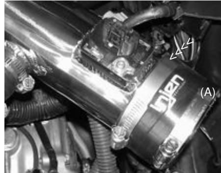
Press the 3" straight hose over the end of intake and tighten clamp located on the intake side. Set clamp on the other side with out tightening the clamp (A).
