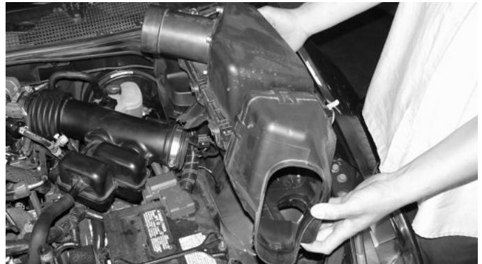
Loosen and clamps and bolts and remove the stock air intake box as shown above.
