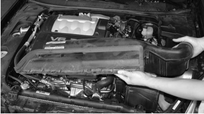
Remove the front air scoop laying over the radiator.
