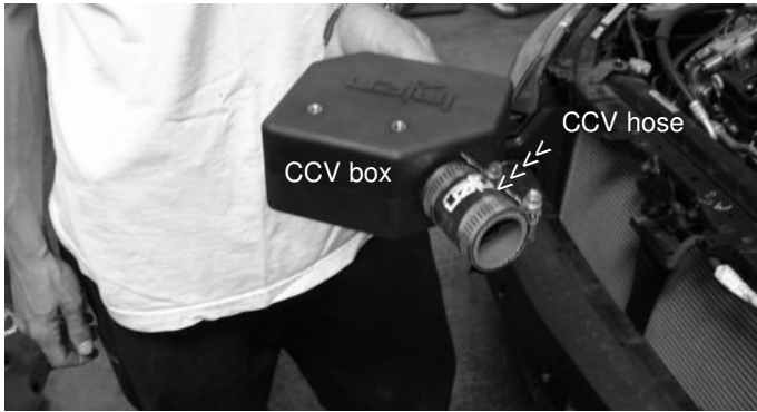
Insert the 1 1/8" CCV hose over the CCV box large port. Use the small clamps to secure the hose in place, tighten the clamp on the port at this time.
