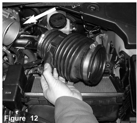
Figure 12 Now, the air intake duct is pulled away from the throttle body.
