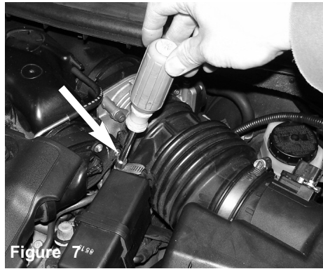
Figure 7 The small clamp on the CCV box is now loosened as shown above.
