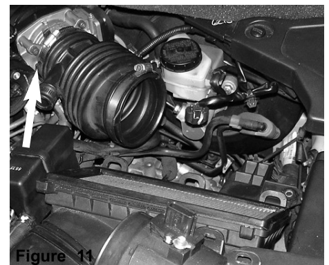
Figure 11 The upper air box is now separated from the lower air box cleaner.
