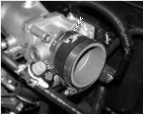
Slip the 2 1/2" straight hose over the throttle body and use two .312 power-bands as shown above. Tighten the clamp that is on the throttle body side.
