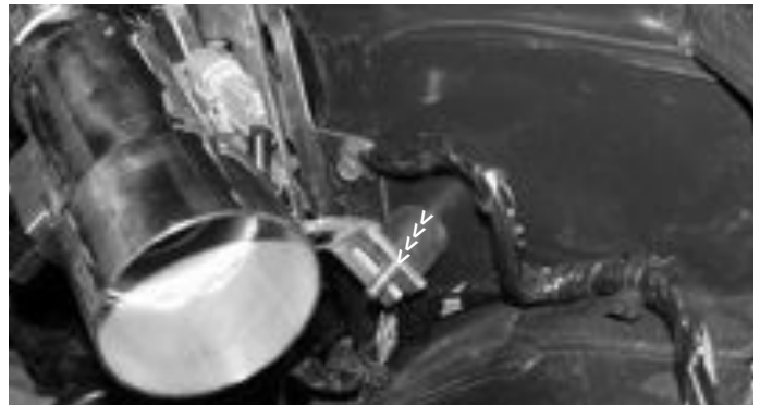
The air intake bracket is shown lined up with the vibra-mount stud and sitting flush on each other.
