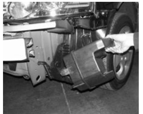
Remove any bolts from the air resonator box then continue to remove the air resonator box as shown above.
