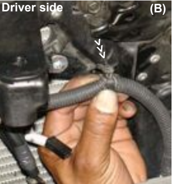
Figure 25 Depress the plastic tab and separate the male and female harness clips (A), pull the male clip away from the crossmember, this will allow the harness to be extended (C). Pull the plastic clip on the wire loom from the crossmember to allow wire harness to be extended further down into the bumper area (B).
