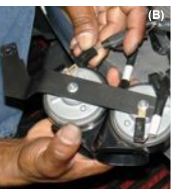
Figure 29 The second horn is aligned and attached to the top of the new bracket, the nut is used to secure the horn in place (A). The electrical wires are reconnected as shown above (B).
