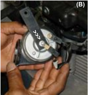
Figure 27 The 10mm bolt on the driver side horn bracket is removed (A). The electrical wires are disconnected from the driver side horn, the nut is also removed in order to separate the horn from the bracket (B).
