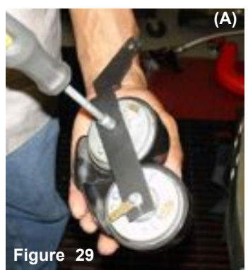
Figure 29 The second horn is aligned and attached to the top of the new bracket, the nut is used to secure the horn in place (A). The electrical wires are reconnected as shown above (B).
