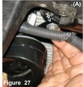
Figure 27 The 10mm bolt on the driver side horn bracket is removed (A). The electrical wires are disconnected from the driver side horn, the nut is also removed in order to separate the horn from the bracket (B).
