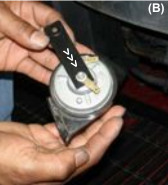
Figure 26 Remove the 10mm bolt holding the passenger side horn (A) The electrical wires are disconnected from the passenger side horn, the nut is also removed in order to separate the horn from the bracket (B).
