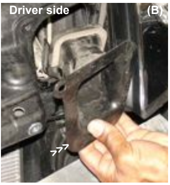
Figure 23 Remove the plastic clips from the front air scoops which are located in front of the passenger side (A) and the driver side (B) cross member.
