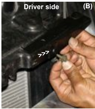
Figure 22 Remove the 10mm bolt from the bumper bracket as shown above. Once the bolt has been removed, continue to remove the brace from the passenger side (A) and driver side (B).
